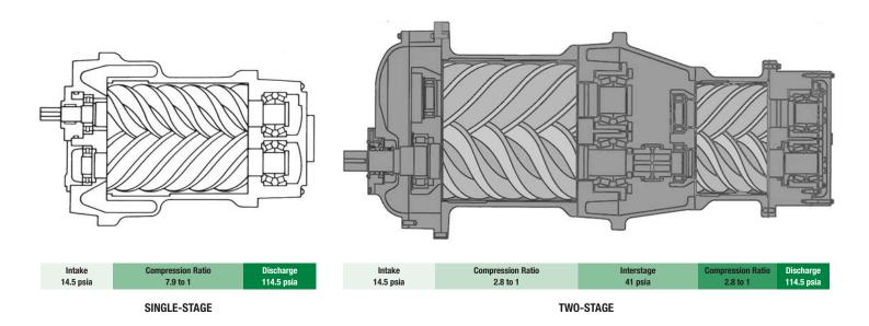
Two-stage compressors\* have a power advantage of 11-13% over equivalent sized single-stage compressors for two key reasons:
