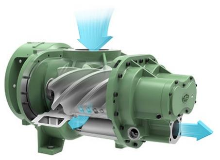
**Turndown** – the turndown ratio refers to the effective operational range of a compressor. The design of a rotary screw compressor relies on pressure and temperatures to operate in specific ranges. Maintaining these ranges is critical to manage the competing forces of physics including rotor and housing expansion and bearing loads.
