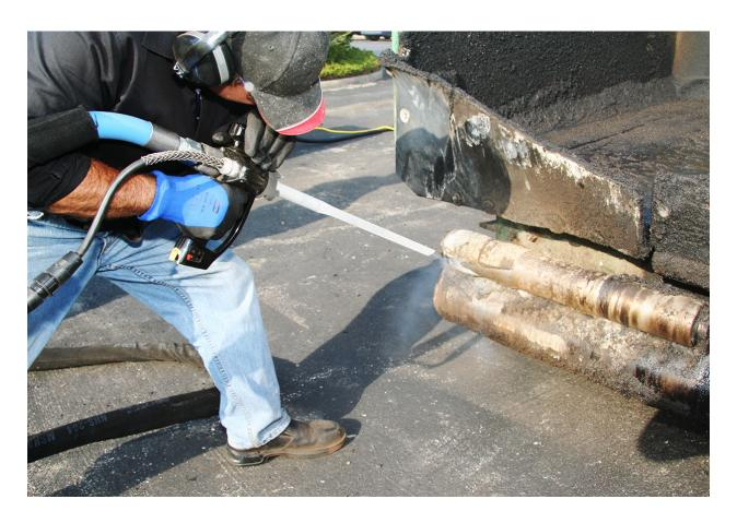
Dry ice blasting, or dry ice cleaning, is a cleaning process that uses media blasting of dry ice pellets to remove contaminants from equipment, tools, surfaces, etc.
